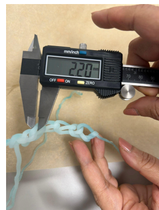
Figure 6- measuring the diameter of the bio yarn using a vernier calliper
